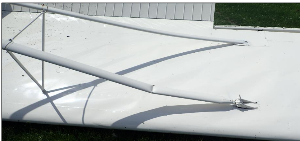
Photo No. 3: Damage to starboard wing strut
