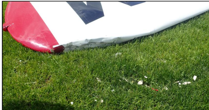
Photo No. 4: Damage to port wing leading edge
