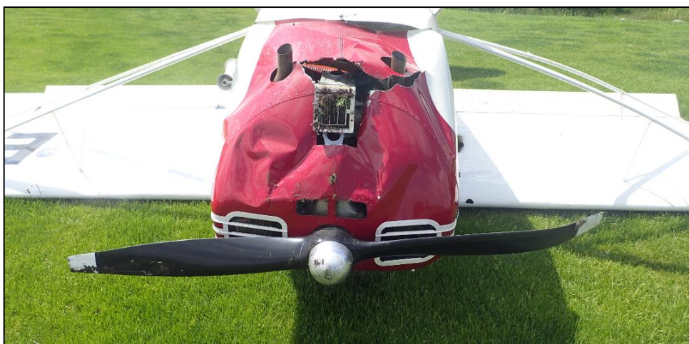
Photo No. 2: Damage to propeller blades and engine fairings
