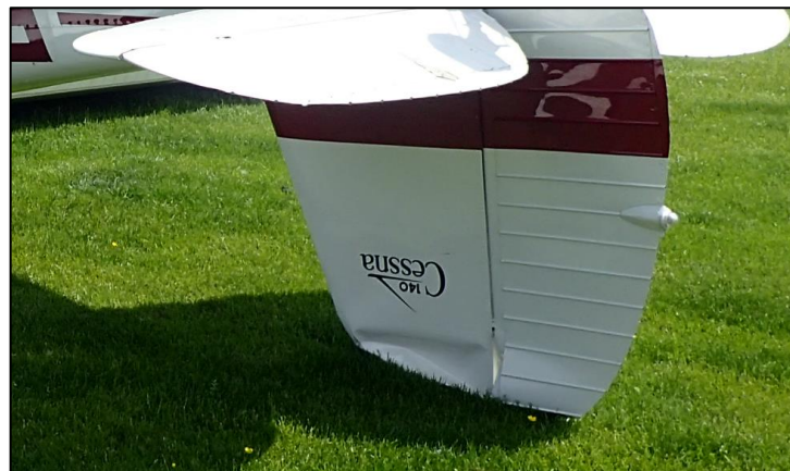
Photo No. 5: Damage to vertical stabiliser and rudder
